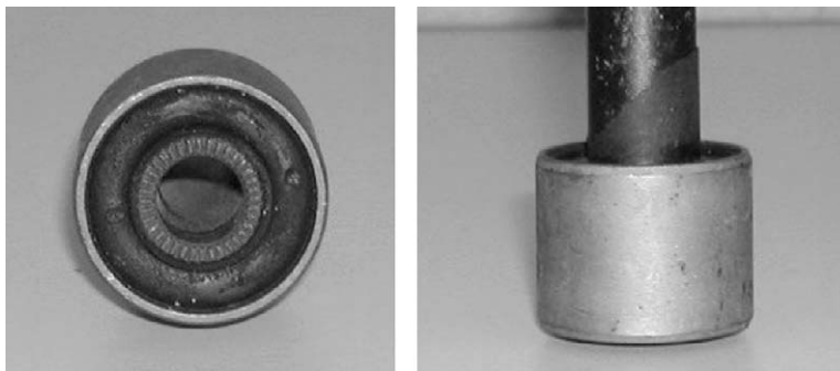
Fig. 9. Picture of the silent-block selected to validate the methodology.
